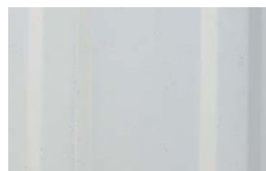
The Frontier Panel exposed to 1,500 hours of accelerated acid rain testing
